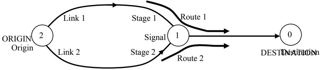
Figure 5. A two route network with two signal stages; link 1 is in stage 1 and link 2 is in stage 2
