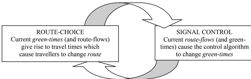
Figure 1. A dynamical system arising when a responsive control system is utilised either in reality or within a model. Current route-flows change green-times (according to some responsive control policy or algorithm) and current green-times generate delays which change route-flows (as travellers seek quicker / cheaper routes). The loop is traversed indefinitely. Here we assume that the dynamical system is to be implemented within a model.
